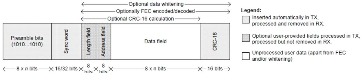
In addition, CC1101 supports fixed packet length protocols, variable packet length protocols and infinite packet length. Details refer to the CC1101 datasheet.
